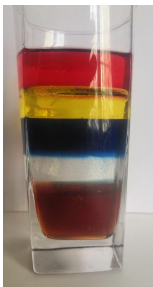
Liquid Tower: (from top to bottom) household alcohol + red colouring, oil, water + blue colouring, washing-up liquid, raspberry cordial.
