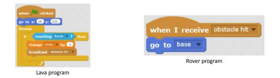
The lava program sends a message to the other programs (especially the rover program). In the rover program, receipt of the message is an event that triggers an action (going to base).
