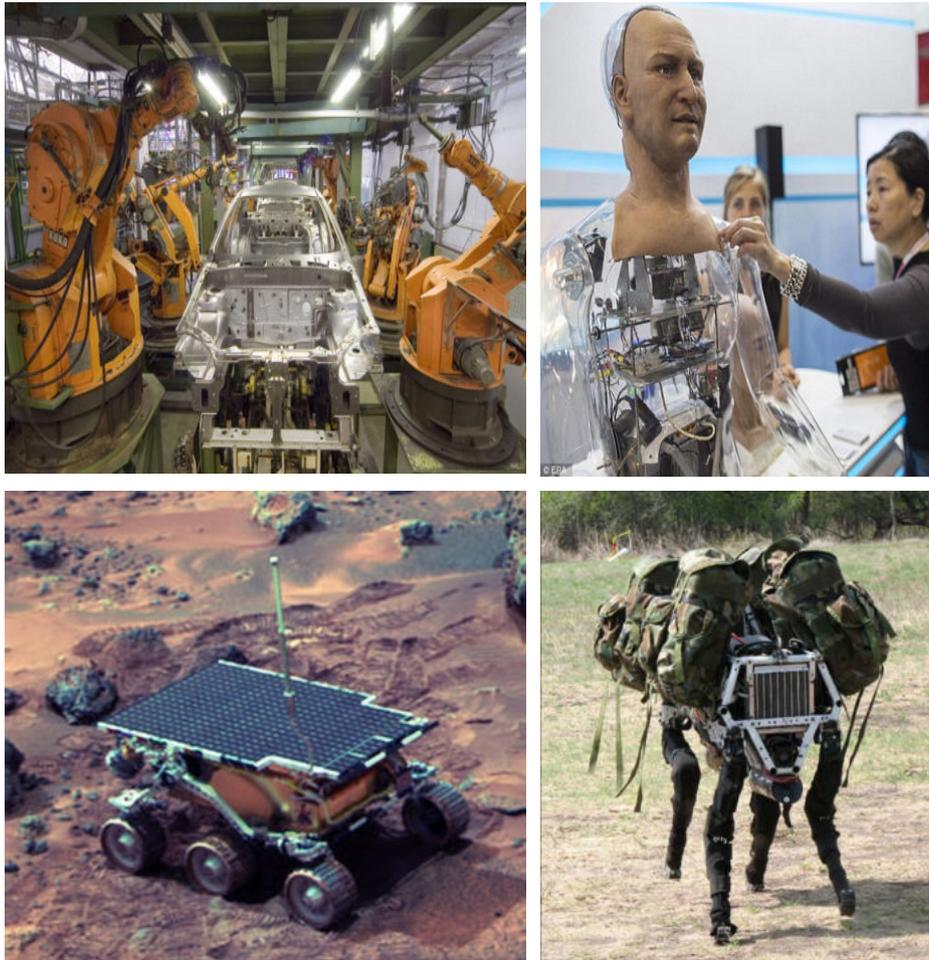
Some examples of robots. From left to right, and top to bottom: mechanical arms used in the automotive industry; humanoid robot designed to recognize and replicate emotions; robot explorer on Mars and military robot designed to carry heavy loads across hilly terrain.
