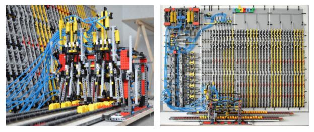
Lego<sup>®</sup> Turing Machine (Rubens project, ENS Lyon): overall view (left) and detail of the reading and writing head (right).
