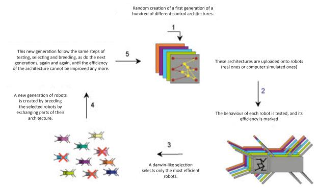
Example of the iterative process that allows "generations" of a robot to learn to perfom a task themselves (for example, movement).
