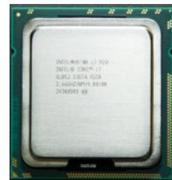
Intel© Core i7 microprocessor from 2014. Contains 2.6 billion transistors.
