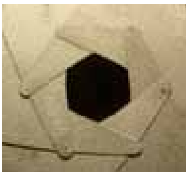
Fig. 6: A six-blade iris from a camera lens
