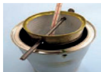
Figure 5.4: Measuring water temperature in the calorimetre.
