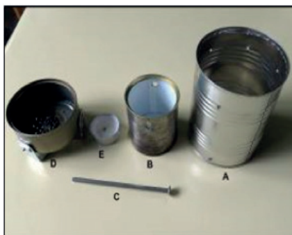
Figure 5.2: Materials to make the calorimeter.
