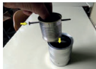
Figure 5.3 A: Assembling the calorimetre.
